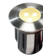
Alpha (4048601) Warm white 0,5 W / 5 lumen Stainless steel 316 46 x 42 mm (H x W x D) Drillhole 30 mm
